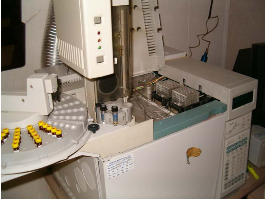
Fort Monmouth, Building 173, Electron Capture Detector Containing Ni-63
