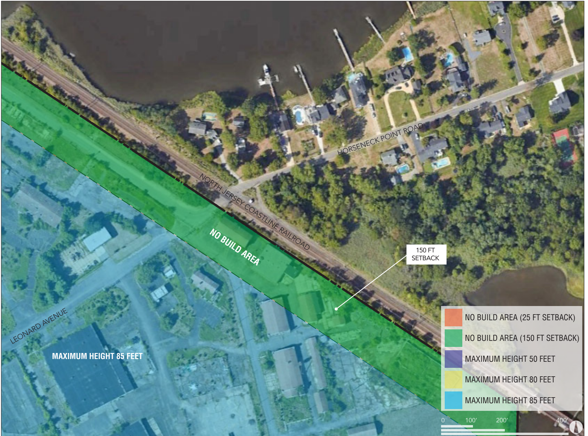
DETAIL OF DEVELOPMENT ZONE 6 HEIGHT REQUIREMENTS ADJACENT TO HORSENECK POINT ROAD | PHILLIPS PREISS GRYGIEL LEHENY HUGHES LLC 2024
